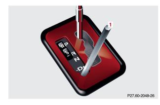
In the case of power failure the transmission selector lever can be manually unlocked, e.g. to tow the vehicle. To do so, insert a pin (1), e.g. ball point pen, into the covered opening below the position "D" of the shift pattern. While pushing the pin down, move selector lever from position "P".
